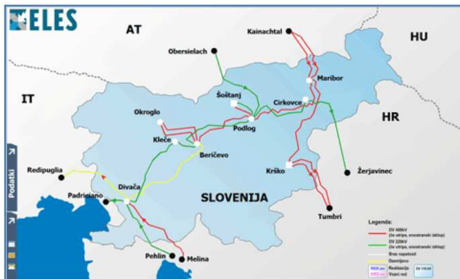
Figure 3: Electric power transmission grid in Slovenia
